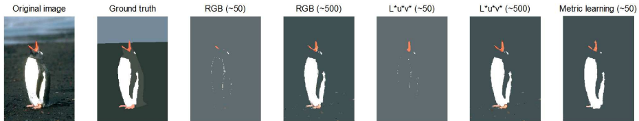
Fig. 4. Segmentation illustration. When the number of clusters is low (around 50), the segmentation provided by RGB or \widehat{L^*u^*v^*} are far from the ground truth, unlike our approach which provides nice results. To get the same perceptual result, both methods require about 500 clusters.
