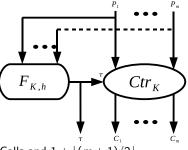
**Computational Cost:** m + 3 Block Cipher Calls and  $1 + \lfloor (m+1)/2 \rfloor$ Multiplications. It increases the ciphertext in 128 bits.
