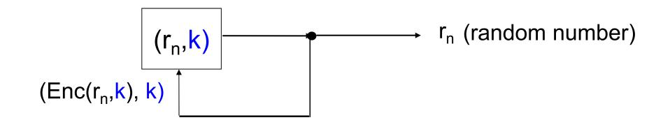
internal state:  $s_n = (r_n, k)$  $s_{n+1} = (Enc (r_n, k), k) =: (r_{n+1}, k)$
