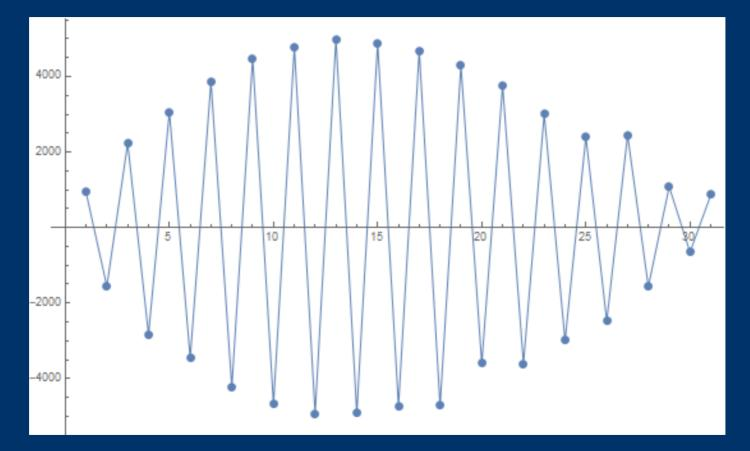
x-axis: subsequent bits, y-axis: difference of 0 bits observed when FF preloaded with 0 or 1
