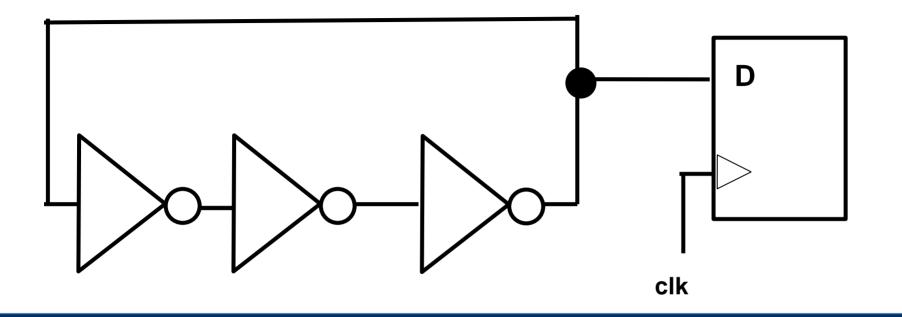
This seems to be a completely trivial and innocent scenario: A ring oscillator is sampled by a D-flip-flop in order to generate random bits.
