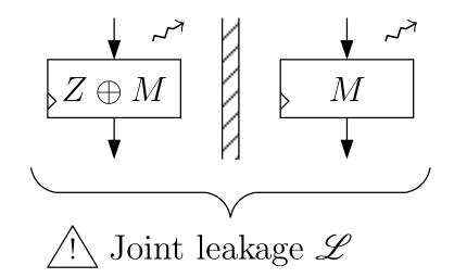
If the leakage is the Hamming weight  $w_H$ , then instead of  $w_H(Z)$ , the attacker will have traces of  $w_H(Z \oplus M) + w_H(M)$ .
