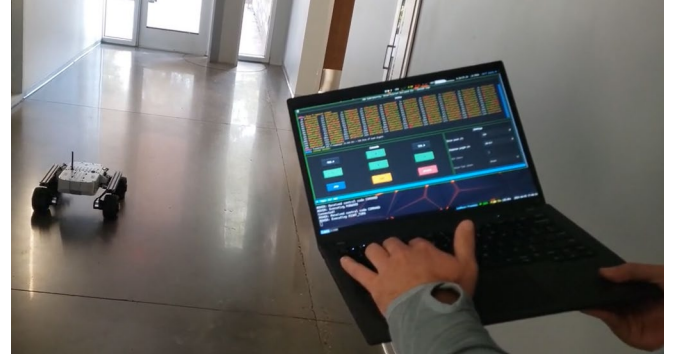
Figure 6. Experimental set up: a PC operating a rover
